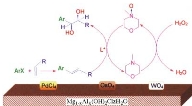
Scheme 1. The catalytic cycle in the LDH-PdOsW-catalyzed synthesis of chiral diols using \text{H}_2\text{O}_2 as the terminal oxidant.
